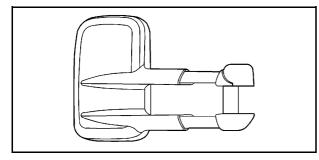
If the vehicle has towing mirrors, they can be adjusted for a clearer view of the objects behind you. Manually pull out the mirror head to extend it for better visibility when towing a trailer.
